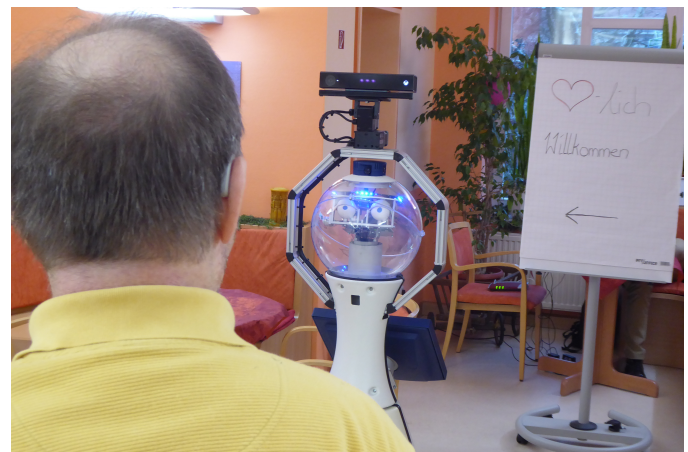
Figure 1: Robot Anna Constantia is greeting a patient to the MAKs therapy. The robot is equipped with an omnidirectional laser range finder, sonar sensors and a Kinect One RGB-D camera. The robots head/eyes has no sensor function.
